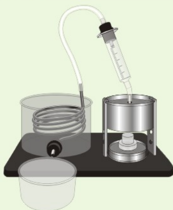
自制物态变化-咸水淡化模型 Self-made state change - salt water desalination model
