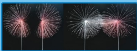
电场线模拟演示器 Electric field line simulation demonstrator
